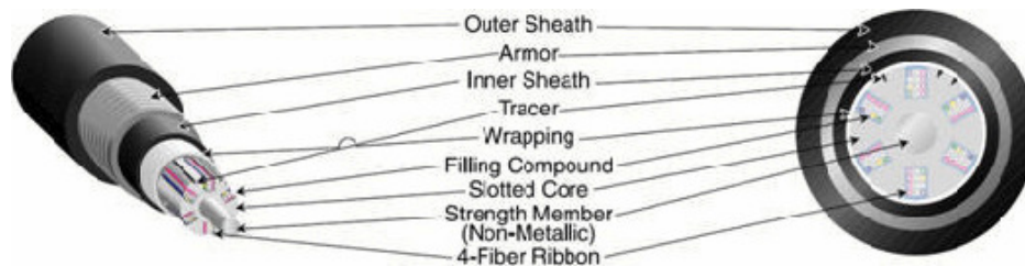
Figure 7-5 : Possible Vertical Fibre Cable design – Ribbon
