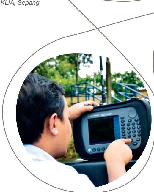
Verification for FM Radio trial transmission reception at Bukit Trig Sandakan, Sabah.
