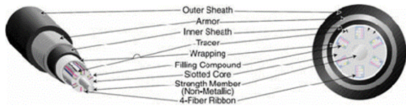
Figure 49. Possible vertical fibre cable design - Ribbon
