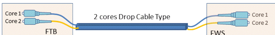
Figure 55. Colour code for 2 cores of drop cable
