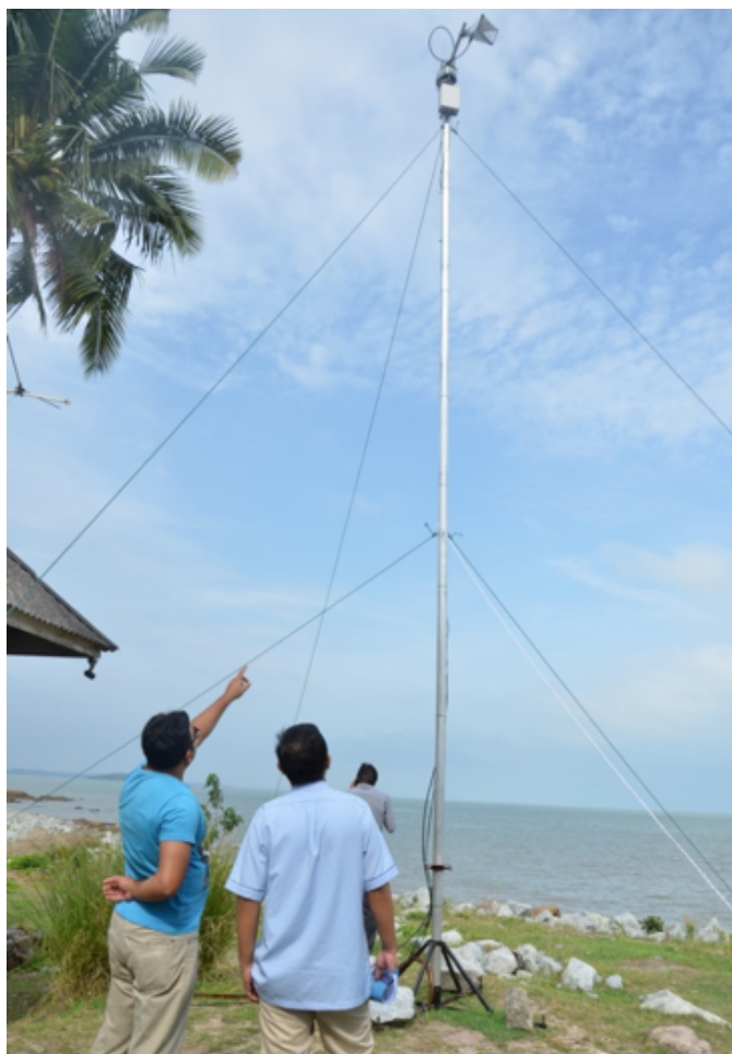
Inspection activities on the experimental transmission equipment for microwave services in the Penyabung Fishermen Village, Johor
