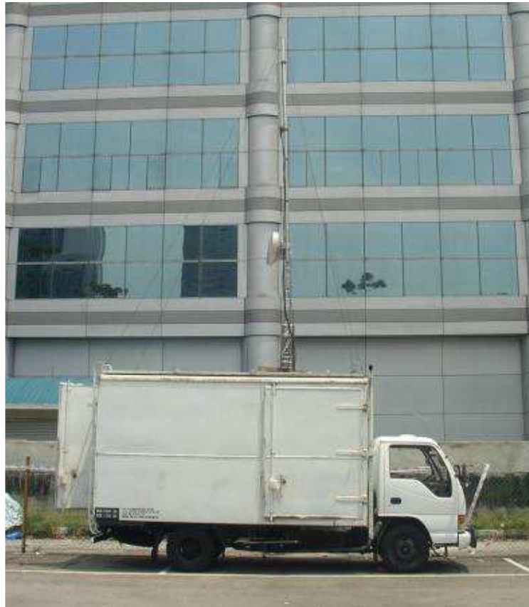
Figure 14. Mobile BTS showing the use of the retractable mini-mast stabilized with guy-wires.
